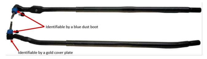
For recalled ACDelco right outer tie rod ends still in your parts inventory, please follow parts return procedures as described in ACDelco bulletin 18D-077 dated June 30, 2018. A replacement outer tie rod, part number 45A7140, will be available for ordering in November 2018.
